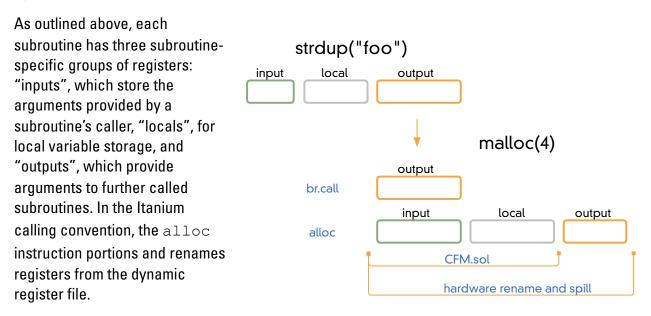
The RSE provides explicit hardware spill and fill. When the dynamic register file is exhausted, the RSE spills GPRs to a region of memory. This memory region can be at a higher privilege level that than the function itself.
